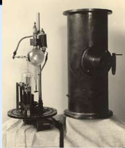
Stebbins-Whitford photoelectric photometer. At left: Kunz photoelectric cell (top) with vacuum tube amplifier (bottom). At right: vacuum chamber, which attaches to the end of a telescope. (UW Astronomy Dept.)
