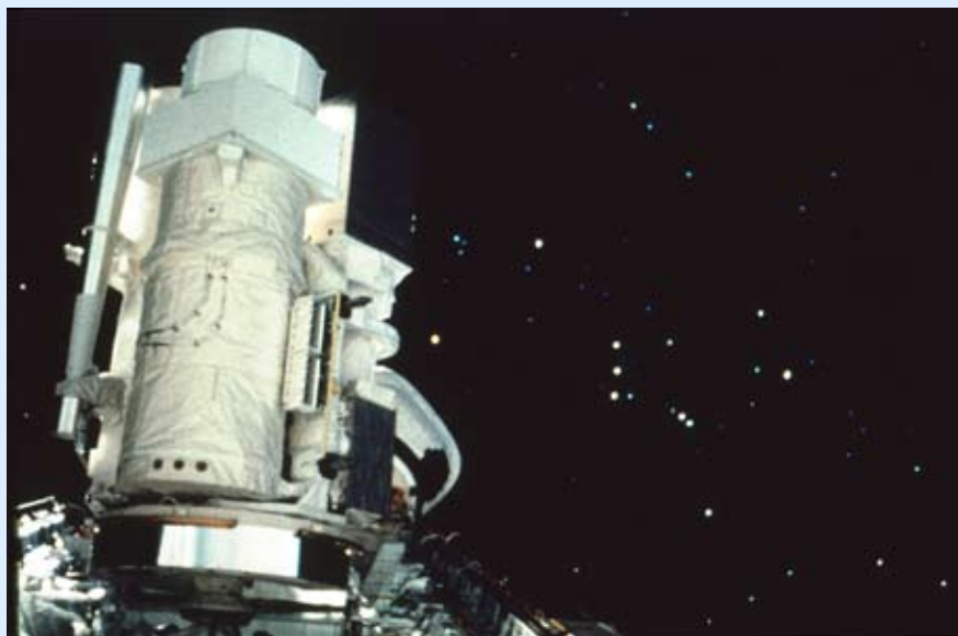
WUPPE and the Astro payload viewed through the space shuttle's payload bay windows with the constellation Orion in the background. WUPPE is the right-most of the instruments in the cluster with its dark, rectangular sunshade near the top. (UW Astronomy Dept.)
