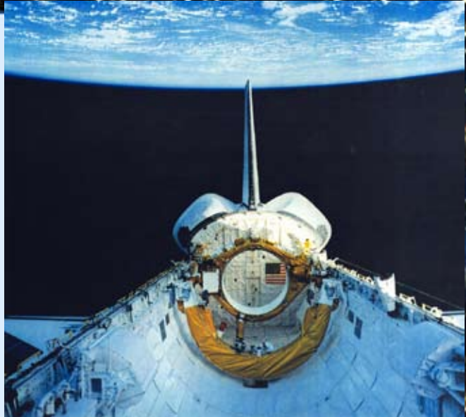
UW-Madison's Diffuse X-ray Spectrometer operating in the cargo bay of the space shuttle. The two halves of DSX are visible at the left and right edges of the cargo bay. (UW Astronomy Dept.)
