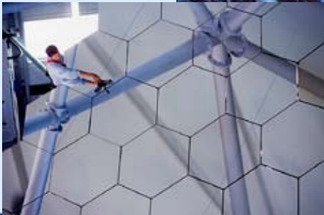
Above: View of the SALT 10-meter mirror through the telescope trusswork with the closed dome aperture visible above. The orange crane is installing the last of the 1-meter mirror segments into the main mirror assembly. Left: The telescope's trusswork is reflected in the mirror's surface. (UW Astronomy Dept./SALT)
