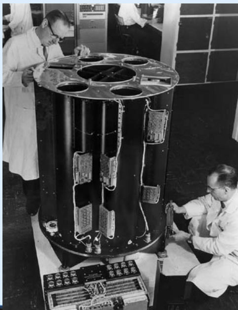
The Wisconsin Experiment Package (WEP), before installation in the spacecraft, being checked by Cook Technology Center engineers. The WEP controller is visible below. (UW Astronomy Dept.)
