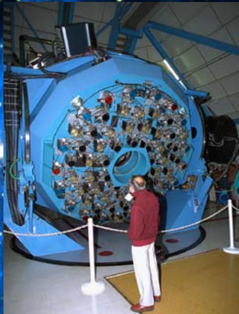
Rear view of the primary mirror housing of the 3.5-meter WIYN telescope showing actuators that adjust the shape of the mirror's surface to perfect its optical performance. (NOAO/AURA/NSF)
