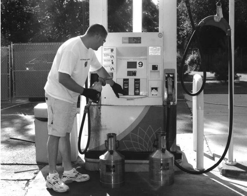
Weights and Measures Inspector Jared Williams tests a gasoline pump to ensure customers receive what they pay for when they buy fuel. (Department of Agriculture, Trade and Consumer Protection)
