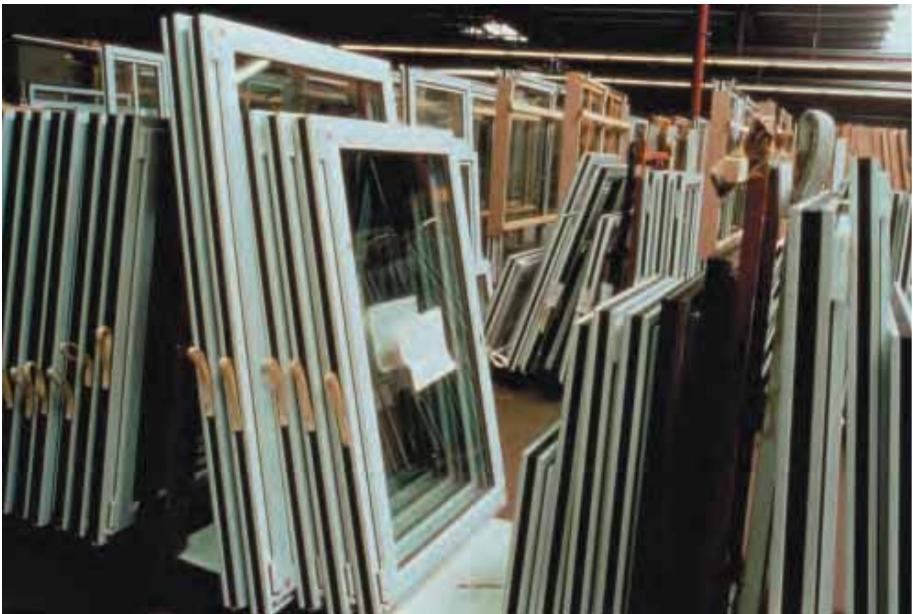
Window profiles from recycled PVC
