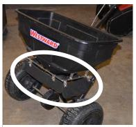
Example of a shield for a spreader to create a narrower spread pattern
