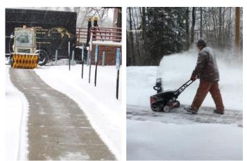
Brooms (left) remove snow closer to the pavement than most other tools (right).
