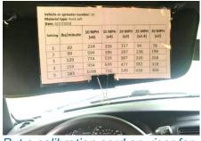
After creating a calibration chart, make one copy for the office and one smaller card for the truck or ATV. Place the card on the visor for easy access. Teach the operator how to use the card in association with the application rate chart. See Chapter 10 for the application rate chart.
