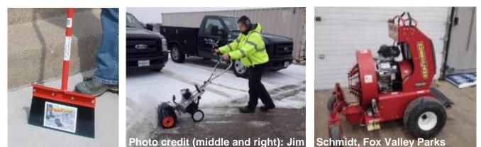
Invest in new and innovative tools to improve mechanical removal and reduce salt. Left to right: flexible scraper, power shovel and riding snow blower
