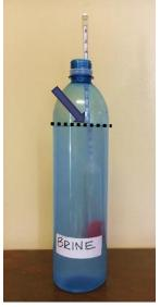
The photo above shows where to read a hydrometer to determine concentration. (marked by the arrow and dotted line)
