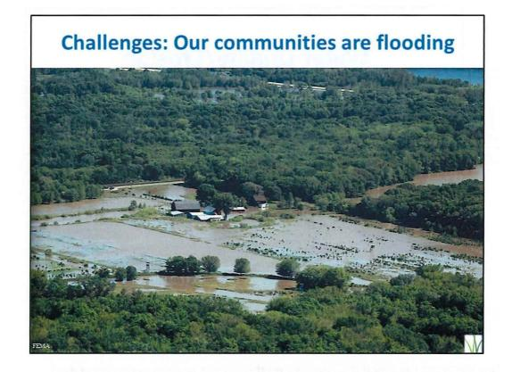
Catastrophic flooding is on the rise. We blame it on intense, localized rain events, but loss of upper watershed wetland and historic floodplain storage increases the damage from these storms.
