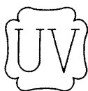
FIG. UG-129.1 OFFICIAL SYMBOL FOR STAMP TO DENOTE THE AMERICAN SOCIETY OF MECHANICAL ENGINEERS' STANDARD FOR PRESSURE RELIEF VALVES
