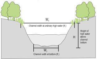
**c2d** CULVERT SIZING. Once the required culvert area has been determined, the applicant can identify the proper culvert size by reviewing the following tables. The minimum size culvert needed to pass flows must have an area that is as much or more than the required culvert area. For example, the recommended culvert size for a culvert area calculation of 8.50 square feet would be 42".
