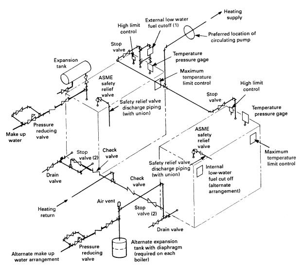
GENERAL NOTE: Plumbing codes may require the installation of a reduced pressure principle backflow preventer on a boiler when the makeup water source is from a potable water supply.
