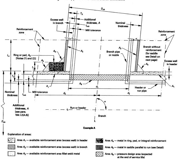
Fig. 104.3.1(D) Reinforcement of Branch Connections
