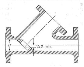
**PG-60.3.7** Shutoff valves, if provided in the pipe connections between a boiler and a water column or between a boiler and the shutoff valves required for the gage glass (PG-60.1.6), shall be of such through-flow construction as to prevent stoppage by deposits of sediment and shall indicate whether they are in open or closed position of the operating mechanism. Some examples of acceptable valves are:
