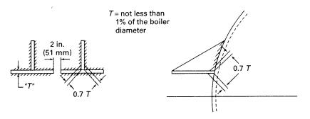
FIG. HG-725(b) WELDED BRACKET CONNECTION FOR HORIZONTAL-RETURN TUBULAR BOILER
