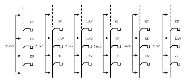
Most restrictive fixture determines stack size
