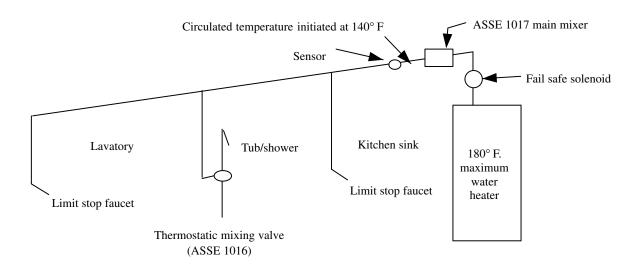
Option 4. Fail safe solenoid provided at main mixer meeting ASSE 1017, combination thermostatic/pressure balance mixing valve meeting ASSE 1016 and limit stop faucets at lavatory and kitchen sink.
