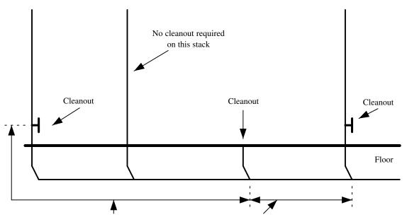
Developed length of drain piping between cleanouts not exceeding 40 feet for 2 inch ID or less, 75 feet for pipe with an ID of greater than 2 inches
