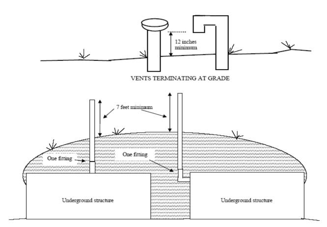
VENTS TERMINATING FOR UNDERGROUND STRUCTURES
