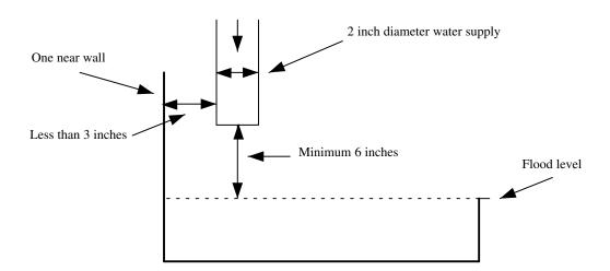
If distance is 3 times or greater than the diameter of water supply (2 inch), then the air-gap is 2 times the diameter of the water supply, (i.e.,  $2 \times 2 = 4$  inches)
