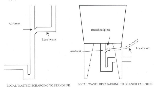
A-382.33 (8) (d)-1. LOCAL WASTE PIPING SERVING WATER HEATER TEMPERATURE AND PRESSURE RELIEF VALVES.
