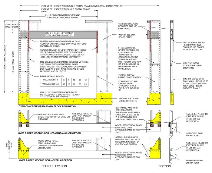
Note: Steel headers are permitted if designed by structural analysis.
