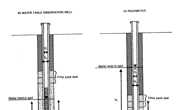
(2) WELLS THAT CAN BE PURGED DRY. All permanent groundwater monitoring wells that can be purged dry shall be developed in a manner which limits agitation by slowly purging the well dry. Wells which can be purged dry may not be surged and no water may be added to the well.
