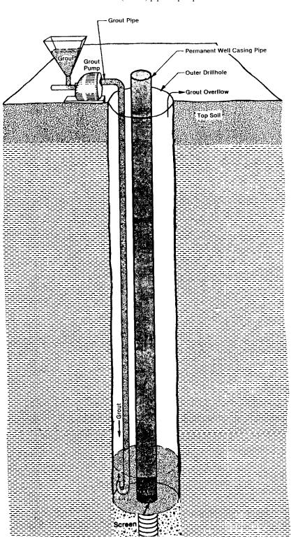
**Figure 3.** Conductor (tremie) pipe — pumped method
