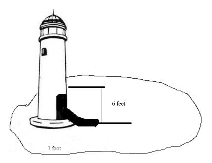
In the drawing above, the obstructed area between the water level to height of 6 feet is 3 square feet. This obstruction would be permitted in a wading pool without a lifeguard plan.
