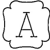
FIG. PG-105.3 OFFICIAL SYMBOL FOR STAMP TO DENOTE THE AMERICAN SOCIETY OF MECHANICAL ENGINEERS' STANDARD FOR WELDED PIPING
