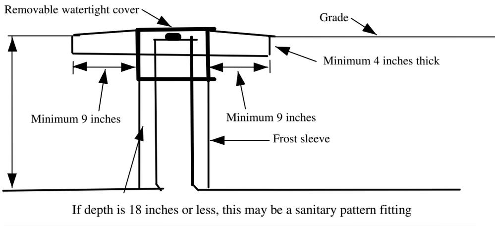
**A-382.35 (8) OUTSIDE DROP INTO AN EXISTING MANHOLE.**
