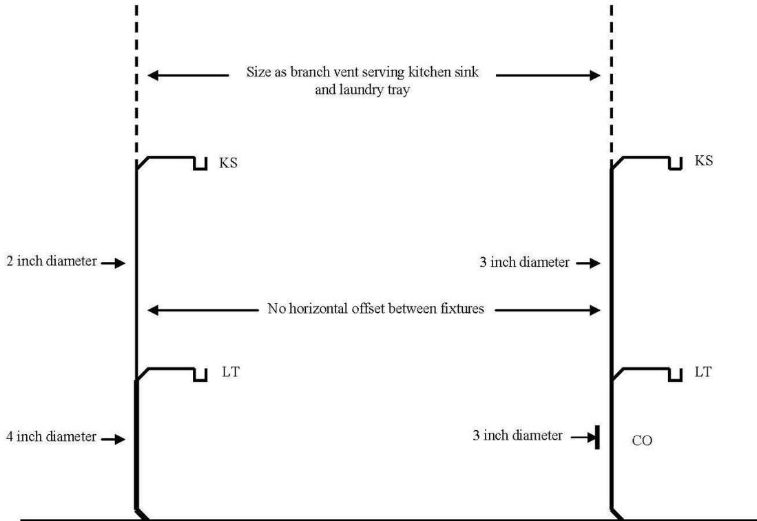
**A-382.31 (17) (b) COMBINATION DRAIN AND VENT BUILDING DRAIN.**
