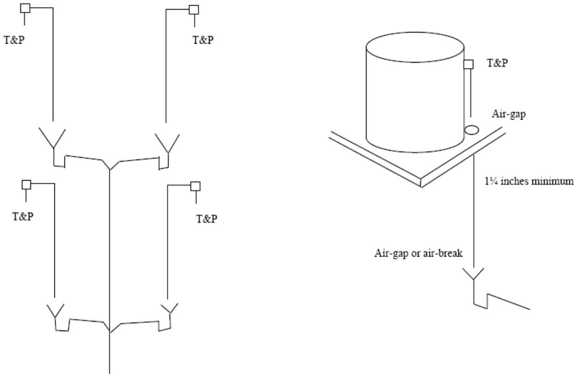
**A-382.33 (9) (c) COMMERCIAL GRAVITY DISCHARGE-TYPE CLOTHES WASHERS.**
