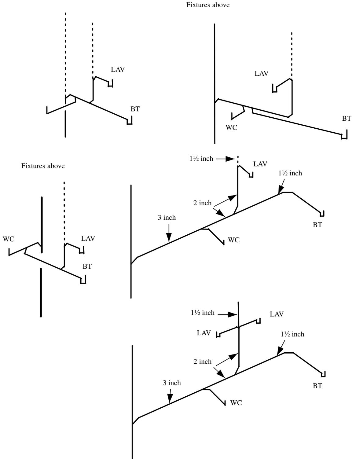
**A-382.31 (13)-2. WET VENTING – FLOOR OUTLET FIXTURES.**
