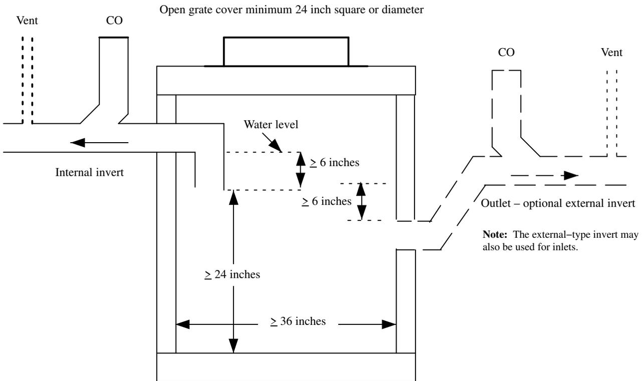
**A-382.34 (4)-2. TRAPPED FIXTURES DISCHARGING TO CATCH BASIN.**
