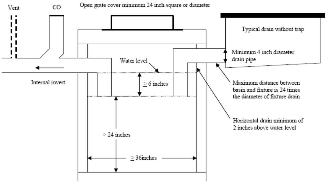
**A-382.34 (4)-5. GARAGE CATCH BASIN WITH FIXTURES ON SEPARATE FLOOR LEVELS.**
