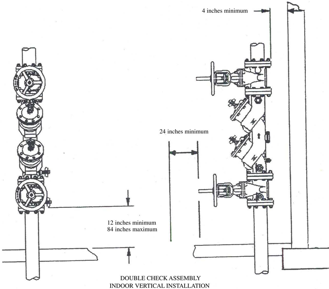
**A-382.41 (5) (f)-5. CROSS CONNECTION CONTROL ASSEMBLY INSTALLATION.**
