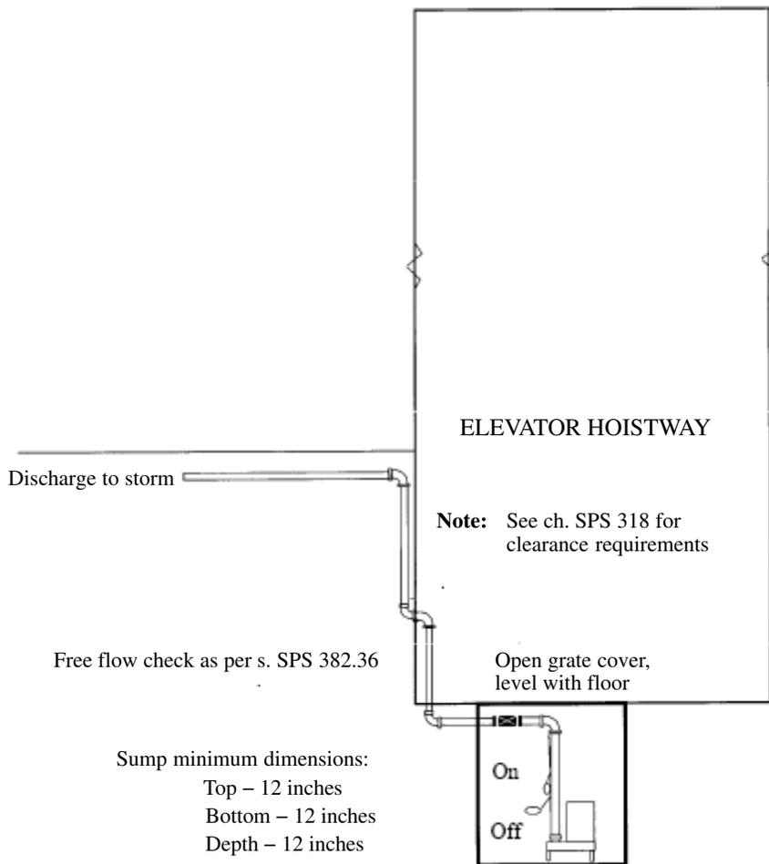
**A-382.33 (9) (f)-2. ELEVATOR PIT SUBSOIL AND FLOOR DRAINS.**
