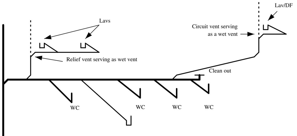
**A-382.31 (14) (a) and (b) SIZING VENT STACKS AND STACK VENTS**
