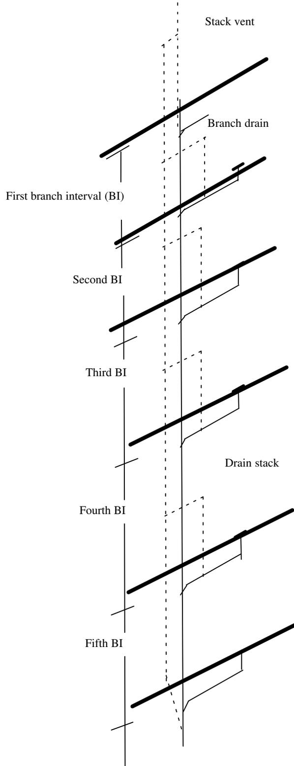
**A-382.31 (4)-2. INSTALLATION OF VENT STACK AND STACK VENT.**
