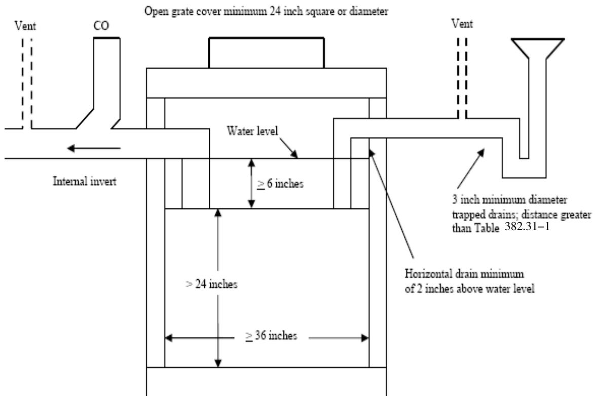
A-382.34 (4)-3. TRAPPED FIXTURE DISCHARGING INTO GARAGE CATCH BASIN.
