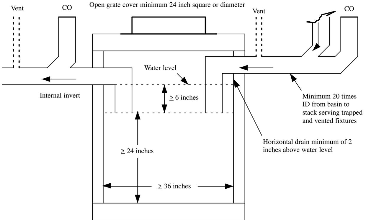
**A-382.34 (4)-6. GARAGE CATCH BASIN RECEIVING PRESSURIZED DRAINS.**
