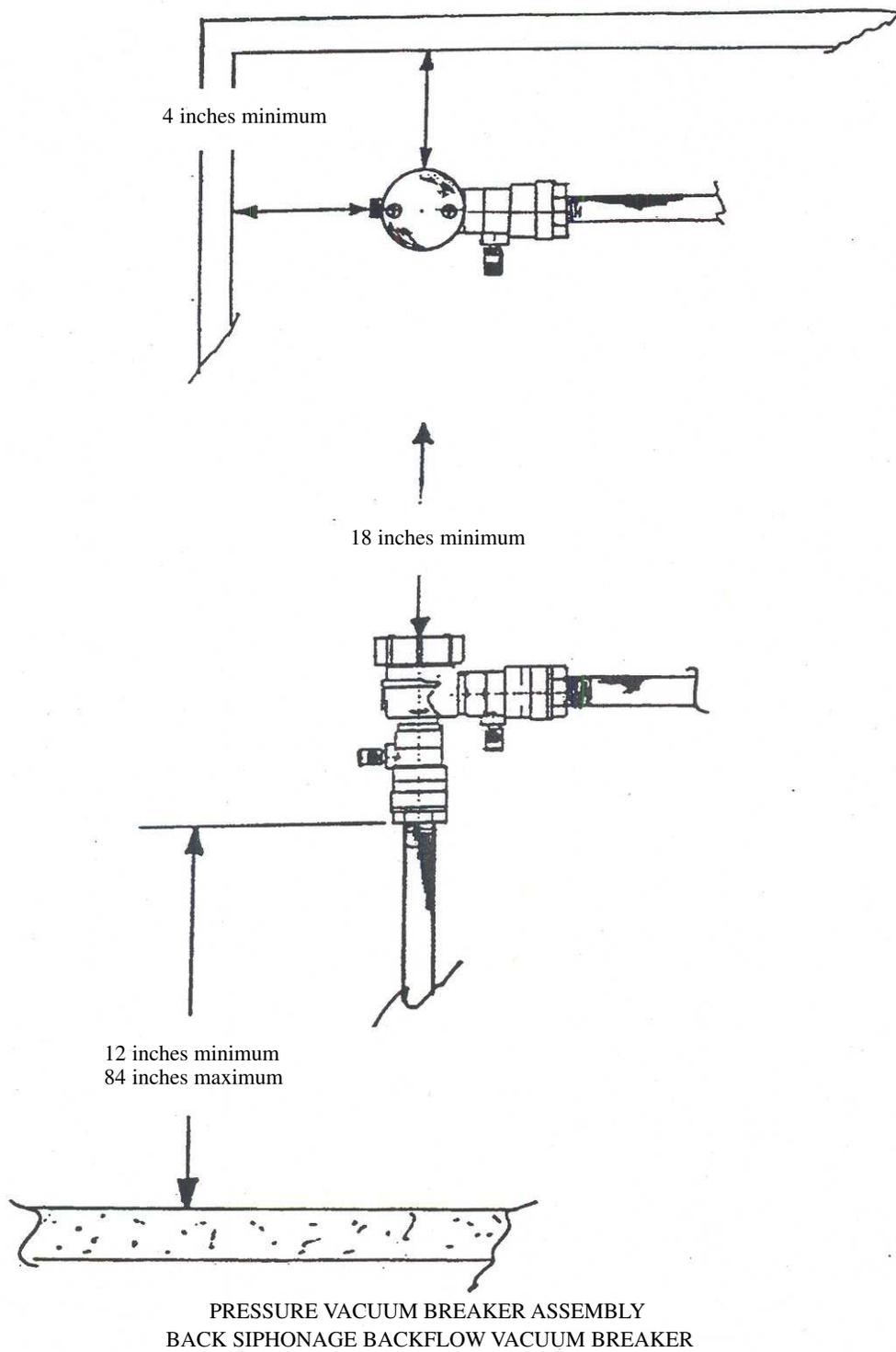
**A-382.41 (5) (f)-4. CROSS CONNECTION CONTROL ASSEMBLY INSTALLATION.**
