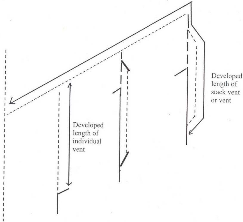
**A-382.31 (14) (c) SIZING BRANCH VENTS SERVING A WET VENT.**
