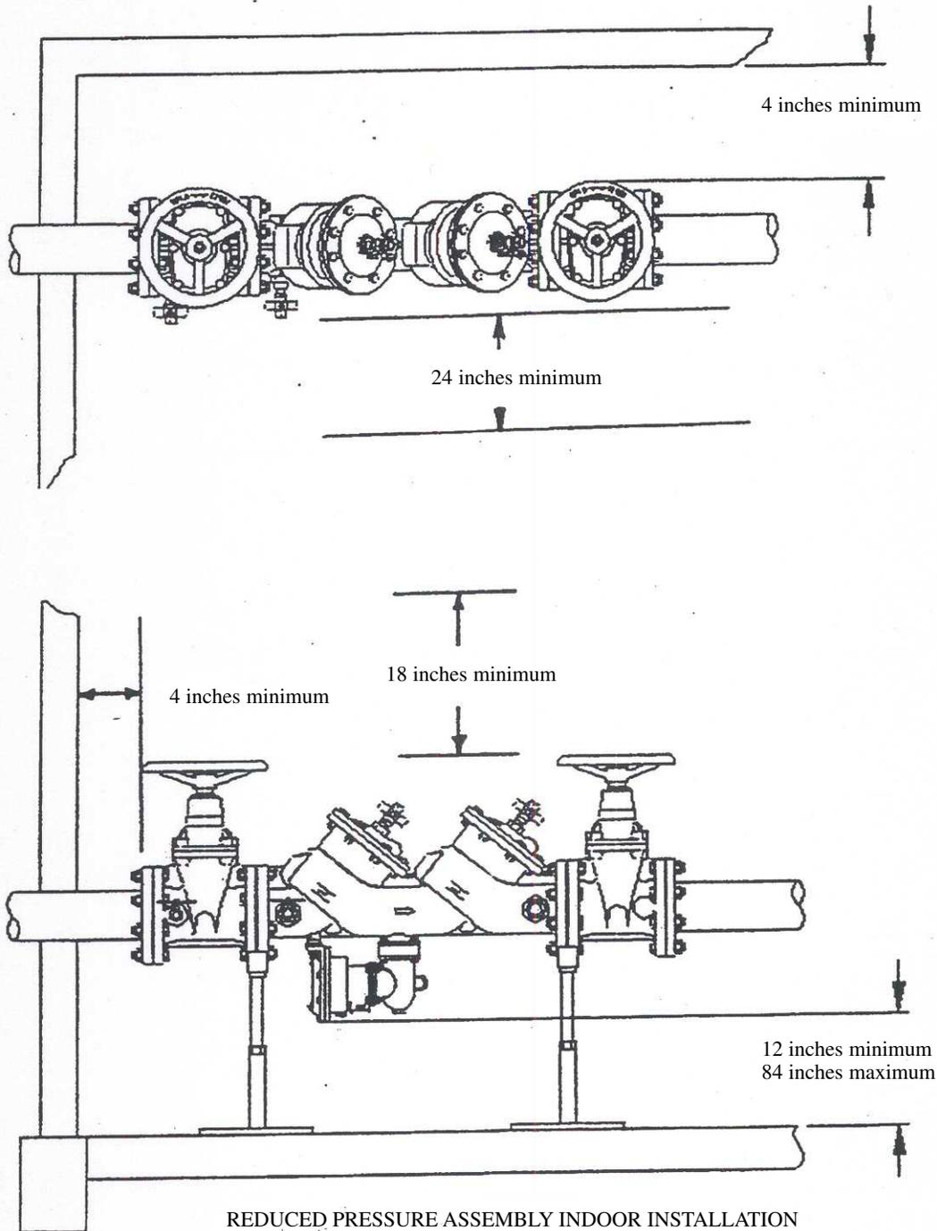
A-382.41 (5) (f)-2. CROSS CONNECTION CONTROL ASSEMBLY INSTALLATION.
