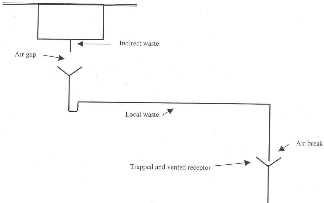
**A-382.33 (8) (a) WASTE SINKS AND STANDPIPES.**
