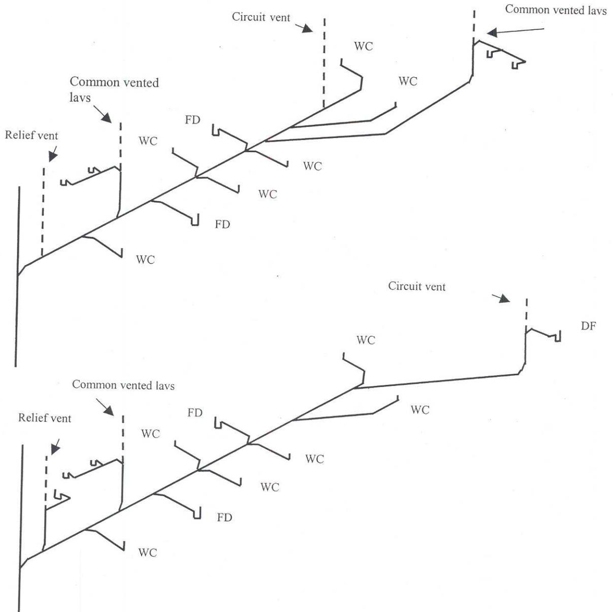
**A-382.31 (11) (a) COMMON VENTS, VERTICAL, SERVING ANY TWO FIXTURES.**
