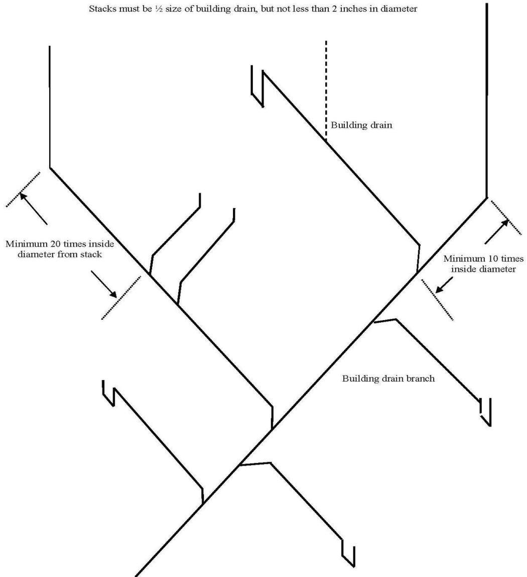
**A-382.31 (17) (c) COMBINATION DRAIN AND VENT LABORATORY SINK VENTING.**
