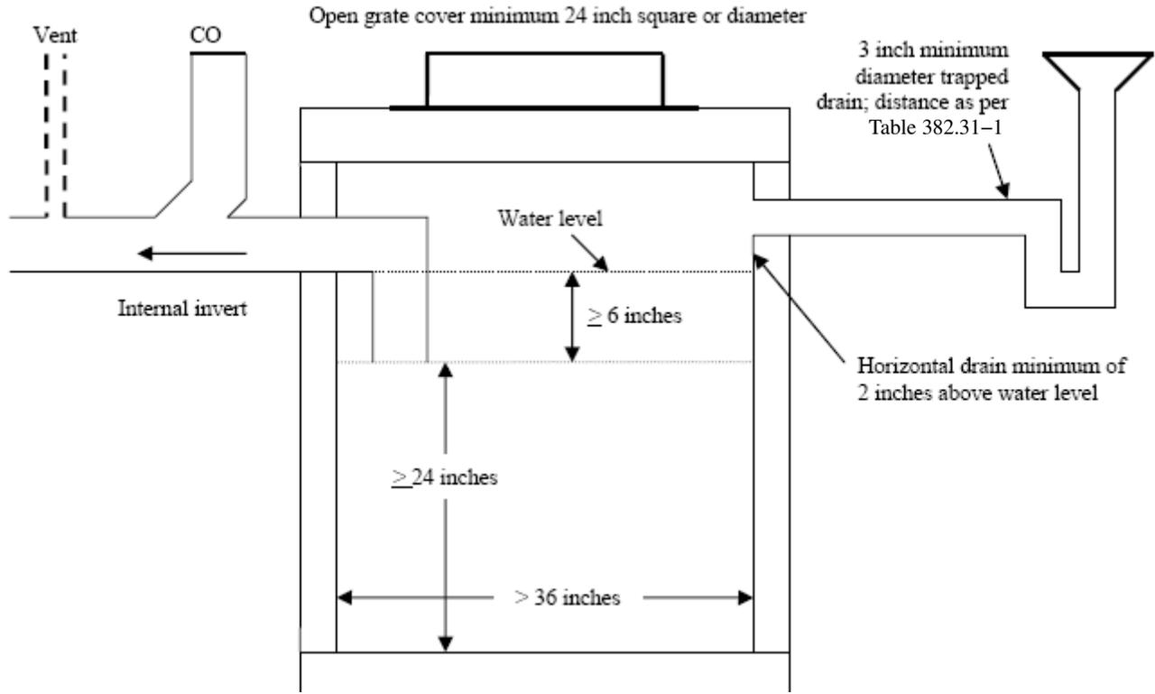
A-382.34 (4)-4. FIXTURES WITHOUT TRAPS DISCHARGING TO CATCH BASIN.
