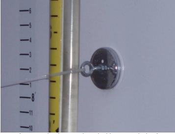
A magnetic plate equipped with an eye-bolt. A wire/cable-tie is then threaded through the eye and tightened snugly around the sight gauge tube.
