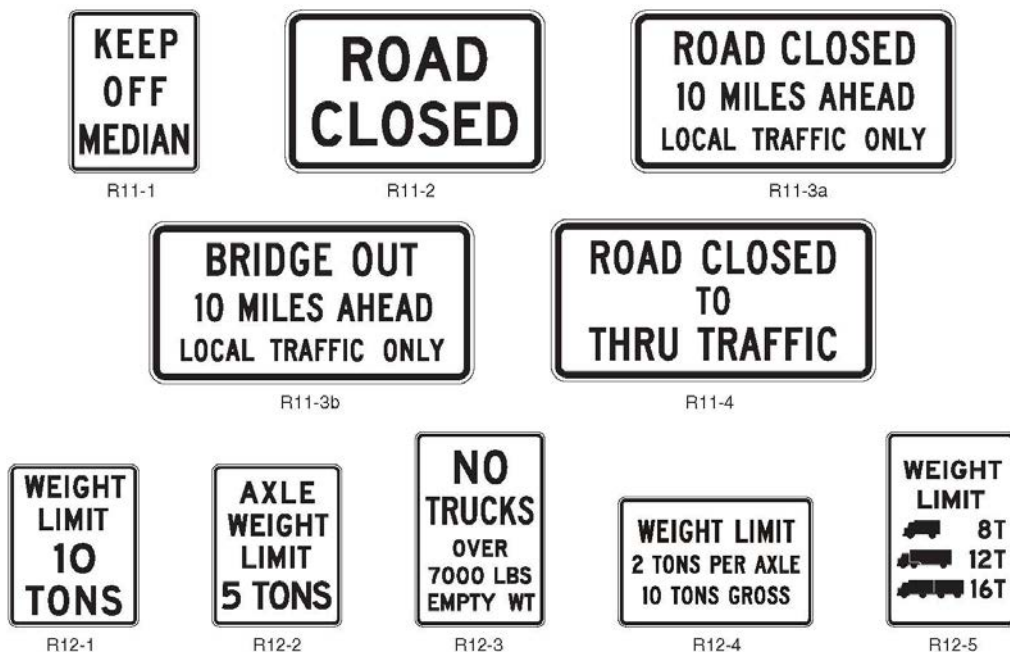
Figure 2B-29. Road Closed and Weight Limit Signs
