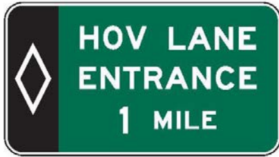
Figure 2G-5. Example of an Overhead Advance Guide Sign for a Preferential Lane Entrance
