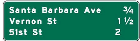
Figure 2E-31. Interchange Sequence Sign
