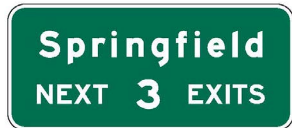
Figure 2E-33. NEXT EXITS Sign
