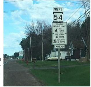
the legal load limit (80,000 pounds) during the seasonal freezing and thawing period. These highway sections have signs posted indicating the allowable weight limits during the period normally
