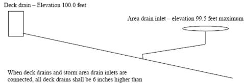
When deck drains and storm area drain inlets are connected, all deck drains shall be 6 inches higher that storm area drain inlets. It must be demonstrated that regardless of the location of any clogged drain, wastewater would discharge from the area drain inlet before ponding on the deck of the pool.
