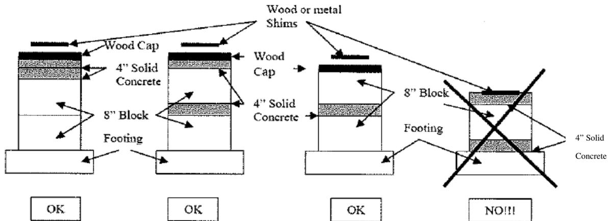
(p) *Footings and foundations.* This is a department requirement in addition to the requirements in 24 CFR 3285.312: Footings and foundations may be designed in accordance with any of the following:
