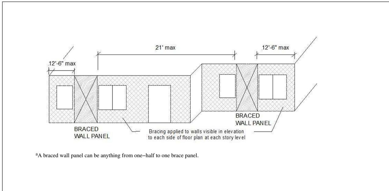
(d) *Braced wall panel support.* Braced wall panels shall be supported on floor framing or foundations as follows:
