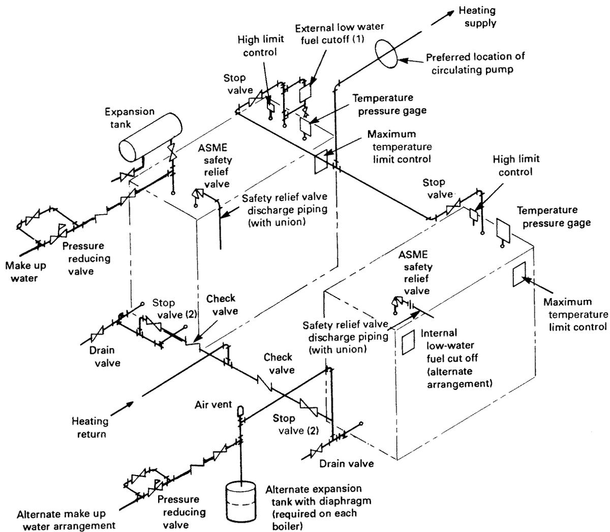
GENERAL NOTE: Plumbing codes may require the installation of a reduced pressure principle backflow preventer on a boiler when the makeup water source is from a potable water supply.
