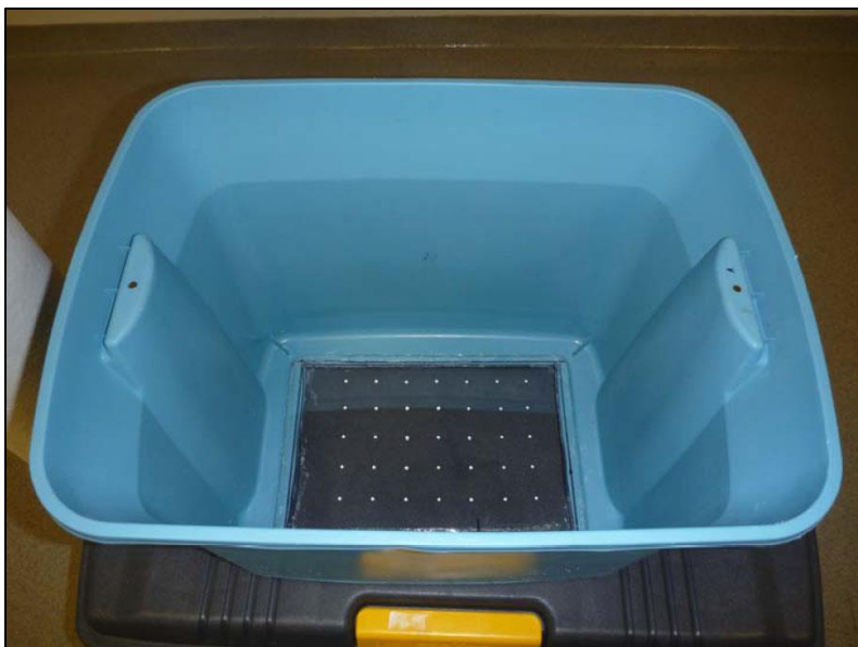
Figure 25. An example viewing bucket from Rhode Island Dept. of Environmental Management. Photograph by A. Patterson.
