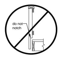
Figure 26 GUARD POST TO END JOIST
