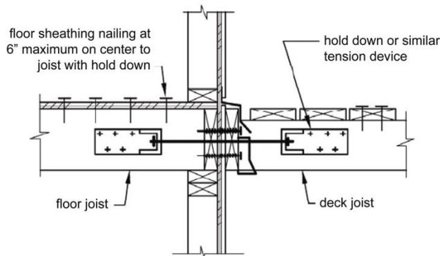
**Hold-down tension devices.** Hold-down tension devices, if used instead of perpendicular bracing as described above, must be provided in at least two locations per deck, and each device must have an allowable-stress-design capacity of at least 1,500 pounds.
