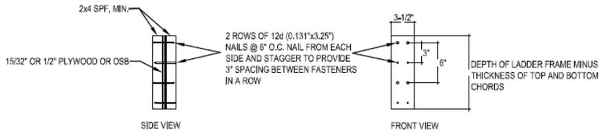
CUT KEY-BLOCKS TO FIT TIGHT BETWEEN TOP AND BOTTOM CHORDS OF LADDER FRAME, INSTALL AT REQUIRED LOCATIONS. ATTACH BLOCKS TO TOP AND BOTTOM CHORDS OF LADDER FRAME WITH 4 - 12d (0.131\"/>
