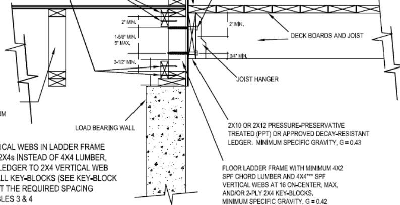
2X10 OR 2X12 PRESSURE-PRESERVATIVE TREATED (PPT) OR APPROVED DECAY-RESISTANT LEDGER. MINIMUM SPECIFIC GRAVITY, G = 0.43
