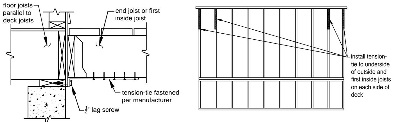
**Tension-tie requirements.** Tension ties, if used instead of perpendicular bracing as described above, must comply with all of the following, but are not permitted for free-standing decks:
