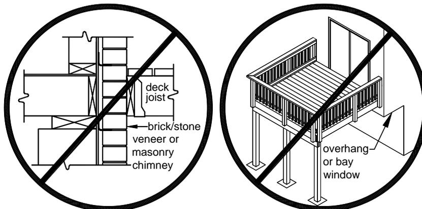
**General requirements.** Ledger board fasteners must be installed in accordance with this section. Placement and spacing must be in accordance with Figure 15 and Table 6. Only the fastener types listed here are approved for use; lead anchors are prohibited. Adequacy of connections may be verified by local inspectors.
