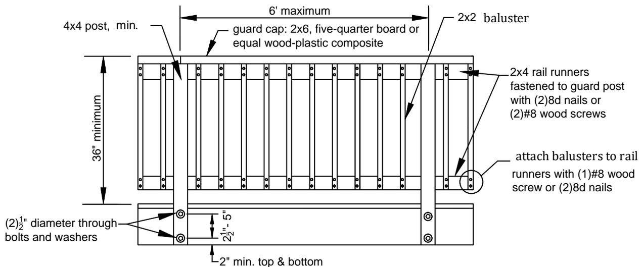
**Guard posts.** Guard posts must be attached to the deck structure in accordance with all of the following:
