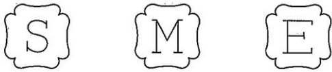
FIG. PG-105.2 OFFICIAL SYMBOL FOR STAMP TO DENOTE THE AMERICAN SOCIETY OF MECHANICAL ENGINEERS' STANDARD FOR ASSEMBLY
