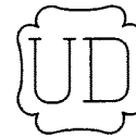
FIG. UG-129.2 OFFICIAL SYMBOL FOR STAMP TO DENOTE THE AMERICAN SOCIETY OF MECHANICAL ENGINEERS' STANDARD FOR RUPTURE DISK DEVICES
