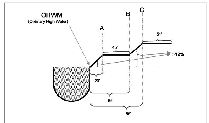
Figure 1: Sample bank determination. In this example the bank extends to C-85 feet.
