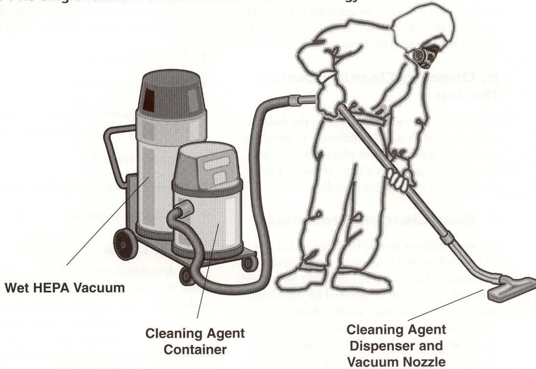
Figure 14.5 Single-Pass HEPA Vacuum/Wet Wash Technology.
