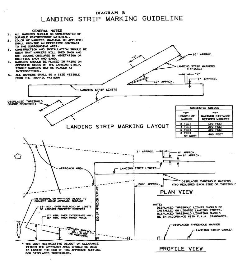
DISPLACED THRESHOLD MARKER LAYOUT
