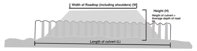
Determining the length of a culvert:
