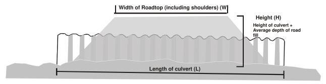
Determining the length of a culvert:
