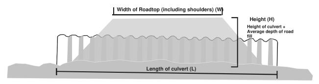
Determining the length of a culvert:
