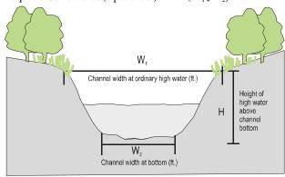
(2) CULVERT SIZING. Once the required culvert area has been determined, the applicant can identify the proper culvert size by
